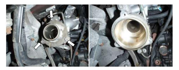
31. Carefully insert your Forge 60mm tapered turbo outlet adapter with new O-ring. Secure with original Allen head bolts. Reuse original O-ring on the outside face.
