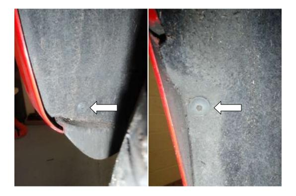
4. Moving to the top of the bumper remove the 4x T25 Torx.
