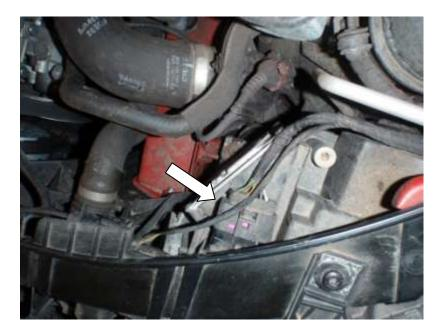
8. To remove the headlights, undo the 2x T30 Torx of the above the headlight. The remaining 2x T30 Torx are located at the rear of the headlight and are slightly more difficult to access.
